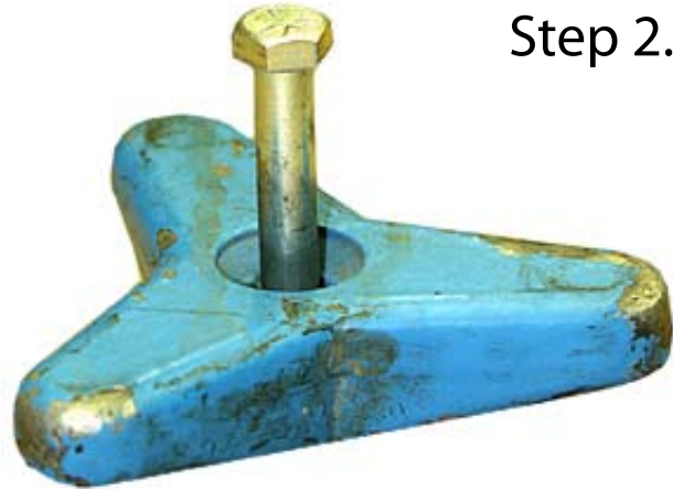
2. Install a new 3/8" diameter bolt by hammering it in the hole. Make sure that it is seated in the casting.
